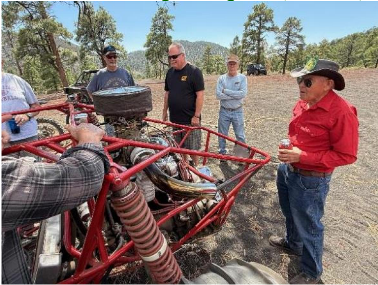
Larry's sand rail weighs in at around 1200lbs and is motivated by a GM small block 383 stroker, so it gets up and goes!
